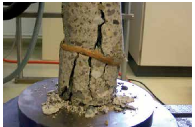
Composite shell lining: crack bridging
