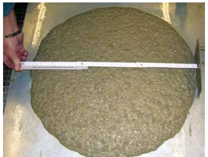
Sprayed concrete quality testing
