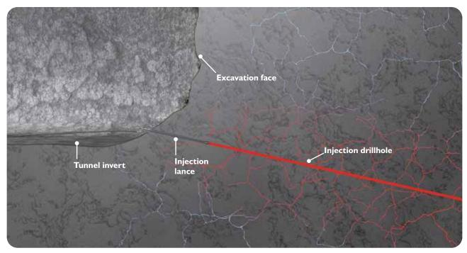
Stable microcement penetrating fine fissures
