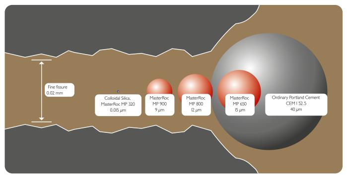
Illustration of the difference in D95 values of MasterRoc MP microcements compared to ordinary Portland Cement
