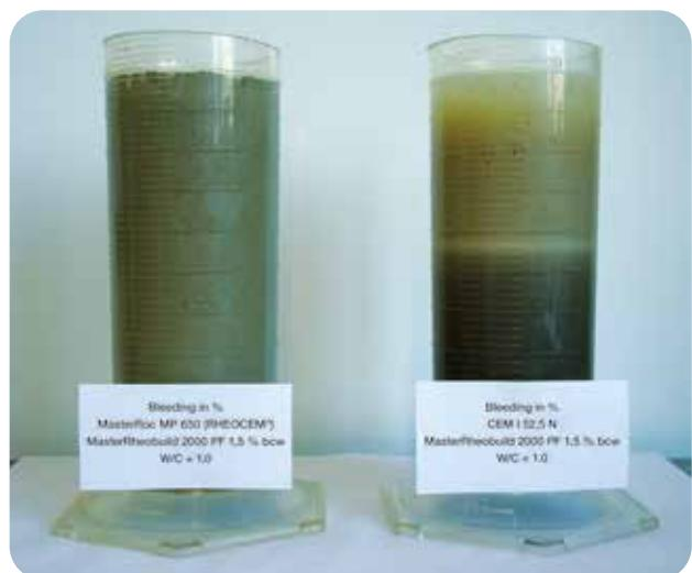
Stable microcement penetrating fine fissures
