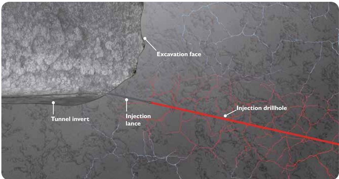
Stable microcement penetrating fine fissures
