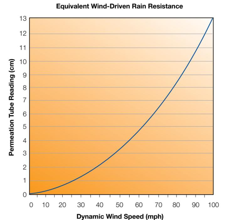
Chart 1: ASTM E 514 Equivalent Wind-Driven Rain Resistance (based on calculated pressures)
