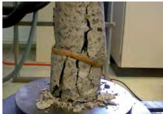
Composite shell lining: crack bridging
