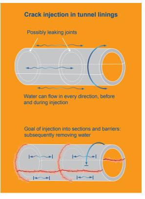
When the underground construction is completed, the ability to swiftly deal with unexpected water ingress and cracks is paramount. We have the right products to help you stop water and make repairs without hassle or delay. Additionally, you can benefit from our acrylics injection products allowing the repair of sheet membrane systems.
