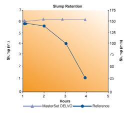
The graphs above are an example of what can be achieved through the addition of MasterSet DELVO admixtures to ready-mixed concrete. The specific dosage for a given concrete mixture will depend on the concrete-making materials and their proportions, the concrete temperature and the stabilization time required.
