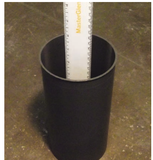
Figure 1. Cylinder mold being used as a measuring device for liquids
