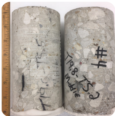
Figure 1 Cores representing concrete with low and expected compressive strength, respectively
