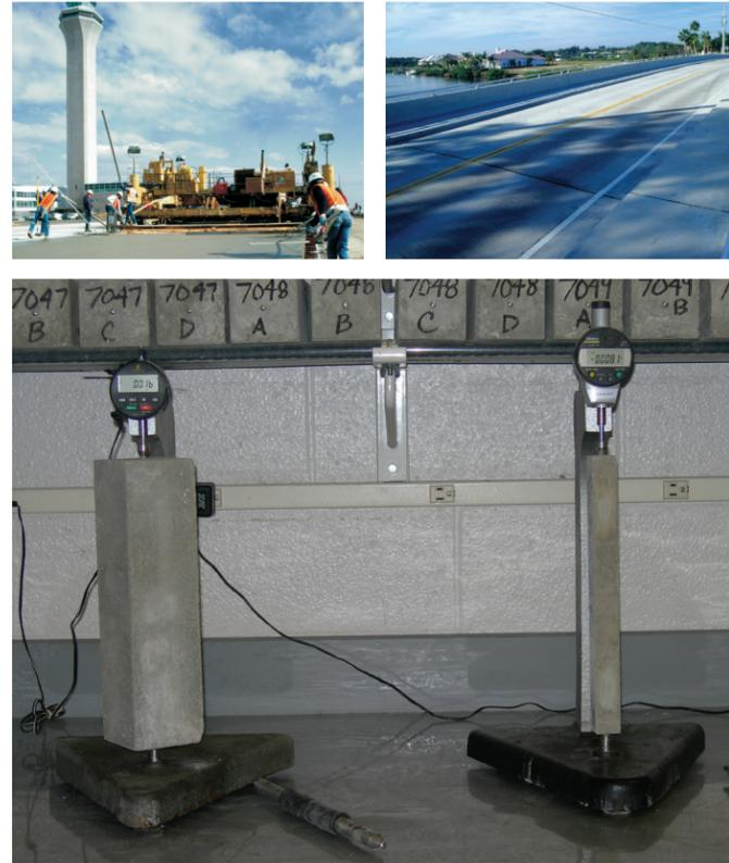
**Figure 3.** Concrete and mortar prisms used in ASTM C 1293 and ASTM C 1260 tests
