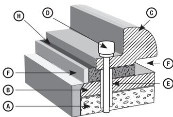
Figure 5 - Typical Epoxy Chock Application
