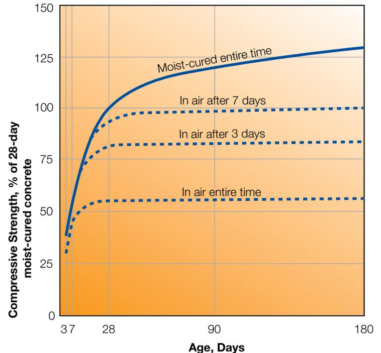
**Figure 4.** Effect of Curing on Compressive Strength of Concrete
