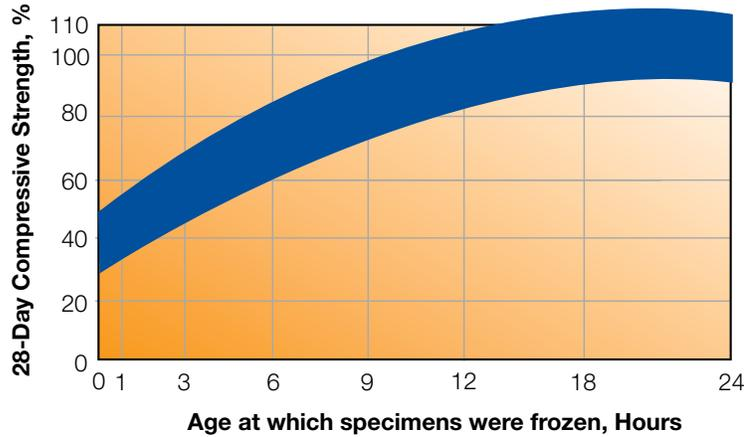
**Figure 2.** Effect of Freezing on 28-Day Compressive Strength of Concrete (Source: ACI Publication SP-39, “Behavior of Concrete Under Temperature Extremes”)
