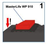
For joint widths from 200mm up to 1000mm, place the MasterLife WP 910 waterbar along the centre of the joint. On wider joint surfaces (greater than 1000mm), two parallel
