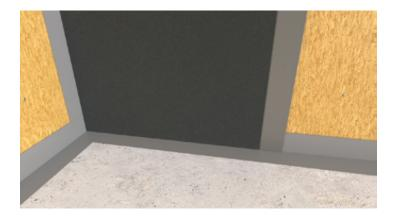
**Method 2:** The MasterLife WP 754 membrane can be folded at the wall floor junction and it is recommended that a fillet it added to this area (MasterLife WP 590, lean mix etc). The corner element can be fully bonded using the MasterLife WP JT waterproofing tape.
