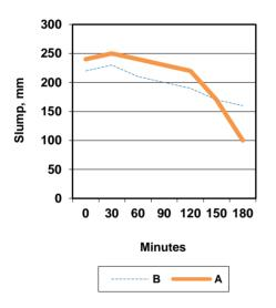
The excellent dispersion effect makes MasterGlenium 27 the ideal admixture for the ready-mix concrete industry. The ability to work with a very low water/cement ratio and still obtain extended workability retention, allows for the manufacture of high quality concrete.
