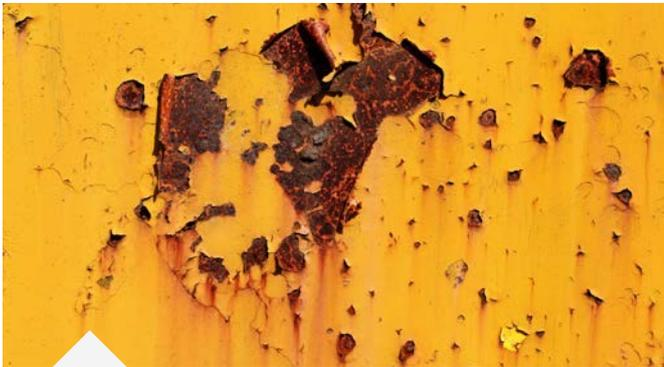
Micro cracks often occur with traditional coatings in areas with special shapes and in the vicinity of the welding of two elements, resulting in corrosion.
