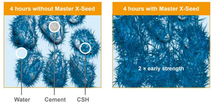
Schematic view of CSH crystals in cement and water pore solution
