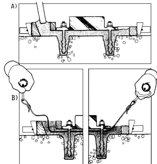
Diagram A illustrates the use of grout surcharge to ensure complete filling under a base. Diagram B shows that straps can be used to aid grout flow under a wider base. A gentle "sawing" action with the strap allows the grout to flow without segregation for greater distances.
