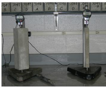
Figure 3. Concrete and mortar prisms used in ASTM C 1293 and ASTM C 1260 tests
