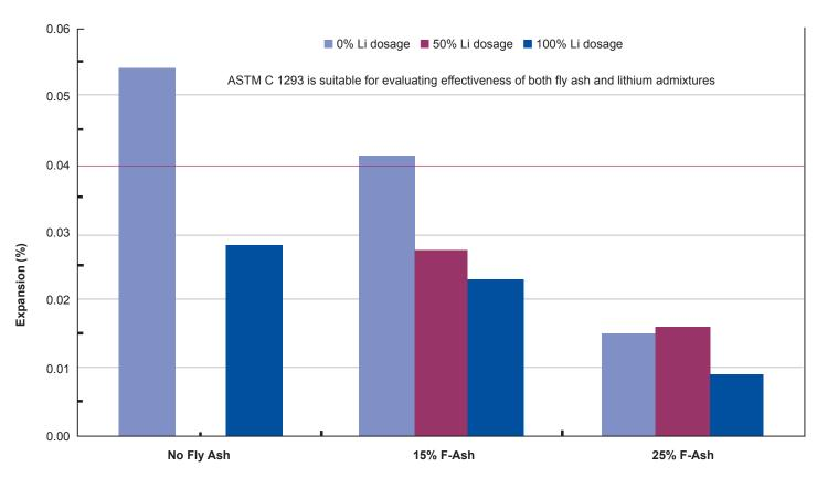
Figure 4. ASTM C 1293 data
