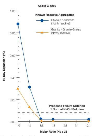
Figure 2. The effect of lithium on controlling expansion caused by ASR (Source: SHRP-C-343, National Research Council, Washington, DC)
